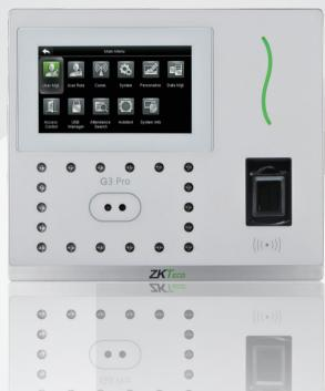
**G3** Pro is powered by Computer Vision technology like 3-in-1 contactless palm recognition, which means the terminal can perform bio-authentication with a user's palm vein, palm print, and the shape of palm at the same time once the sensor detects a hand presented.
